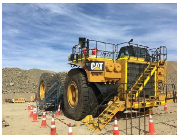
Candelaria new CAT 793F haul truck assembly
